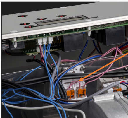
Looped Pink Wire – Fireman's switch connection
