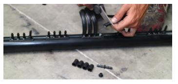
**STEP 1:** Strip the collector back and cut the end of the broken barb just below the joining barb to remove it.
