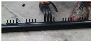
**STEP 5:** Lubricate the hole and insert a joining barb.
