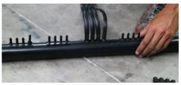
**STEP 8:** Push the pressure sleeve down over the strip to secure.
