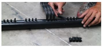
**STEP 4:** Place a grommet into the cleaned hole.
