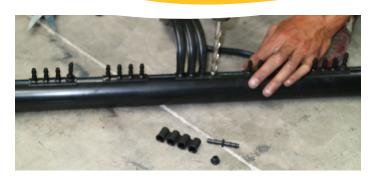
**STEP 2:** Drill out the hole using a 8.5 - 8.7mm drill bit. Be careful if the drill bit is new.
