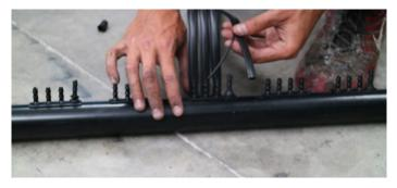
**STEP 6:** Peel the excess collector back to expose a single strip.
