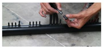
**STEP 7:** Place a pressure sleeve over the strip. Apply a lubricant onto the barb and push the strip onto the barb.
